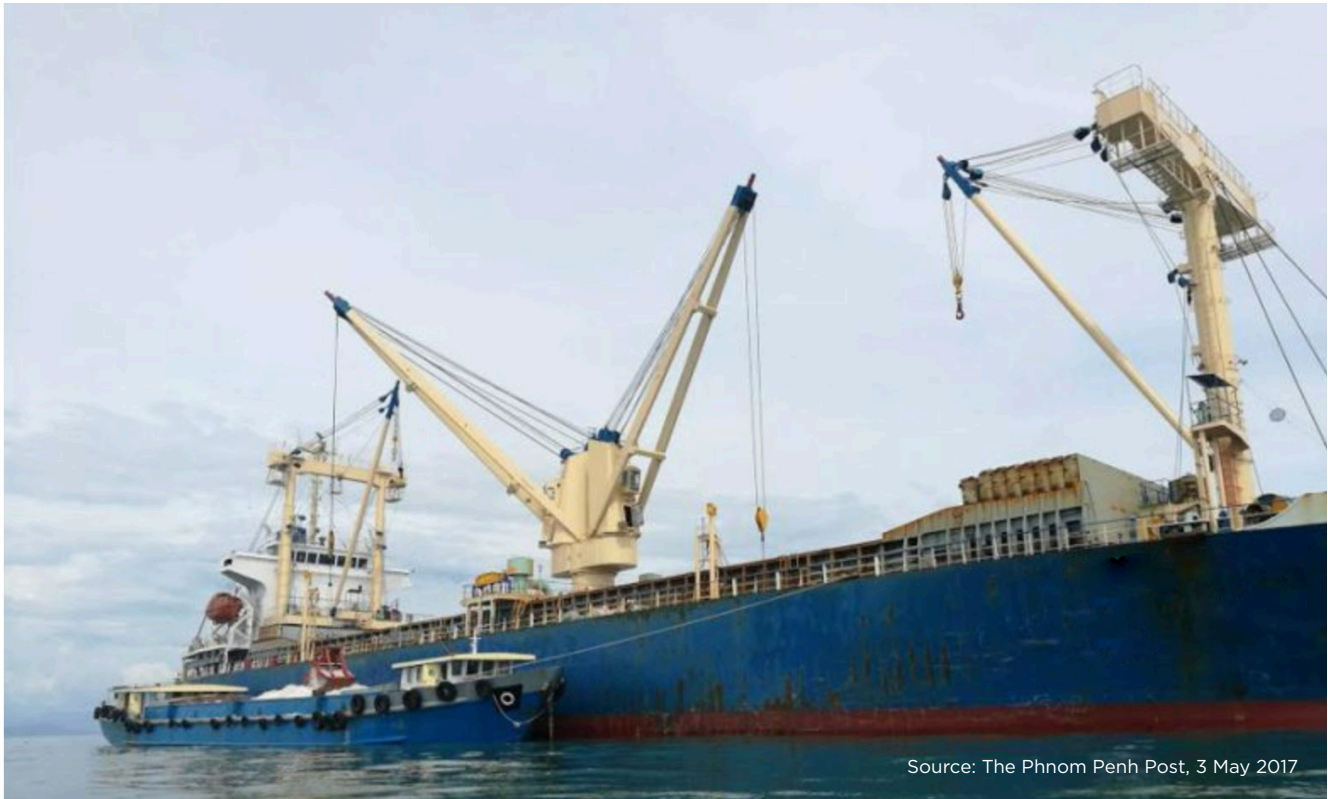
Figure 20: An example of silica sand being loaded from a barge to a bulk carrier using a grab crane
