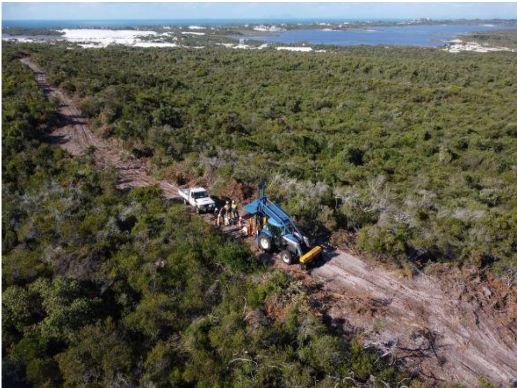
Figure 5. Yearlong Contractors vacuum-based drill rig working at CFS project with Mitsubishi silica sand operations in the background
